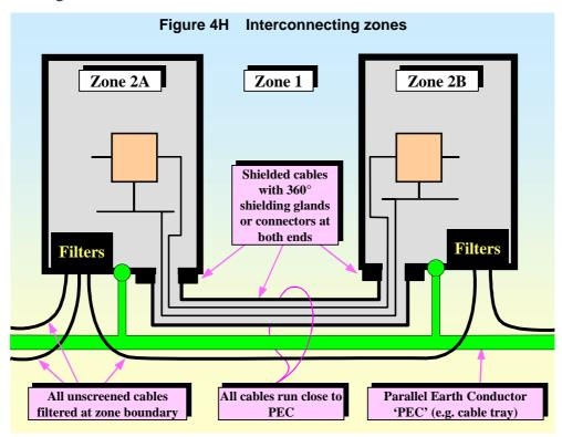
All screened cables that enter or leave shielded zones must have their screens terminated by 360° electrical contacts in shielding glands (or connectors) at the enclosure walls. Where the zone is simply defined by a MESH-CBN, high-frequencies will not be shielded against (depending on mesh size) but still the screened cables must be bonded at the zone boundary, for example by using a saddleclamp to bond them at the filter bonding plate shown in Figure 4E above.
