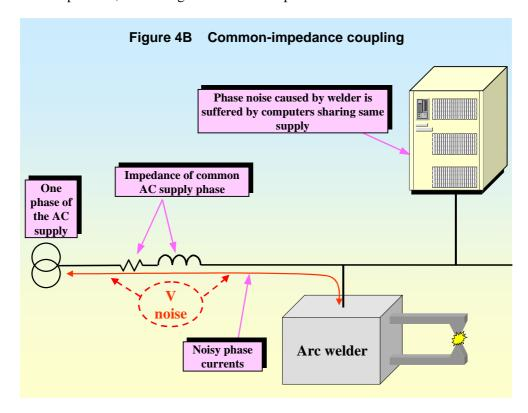
A similar situation occurs in the CBN, but the currents are less predictable as they are mostly caused by 'earth leakage' from mains filters, failing insulation, and motor leakage currents (via stray capacitance from windings to frame). In modern offices, 'earth leakage' due to the RFI filters fitted to computers can be very large indeed. In one recent building 70 Amps of leakage current due to computer RFI filters alone was found at the main earthing terminal [13].
